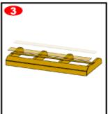
4. Cut four 13-3/4" long uprights from the 2X4 stock and attach them to the bottom back brace already cut from your template. One upright should be placed at either end of the brace, with the space of 15-1/2" between each upright and its mate. Install with glue and 3" screws.
